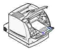
f. Reinstall the toner cartridge. Align the slides on the cartridge with the slots on the toner cartridge cradle. Use the arrows inside the printer for placement. Guide the cartridge in until it *snaps* into place.
