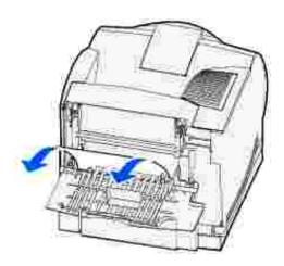
If the print media does not move immediately when you pull, stop pulling. Remove the toner cartridge, and then pull the print media out.
