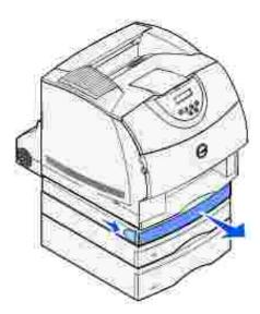
9. If the edge of the print media is visible, pull the print media straight up and out.
