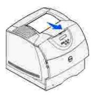
If the print media does not move immediately when you pull, stop pulling. Open the upper front door and pull the print media out.
