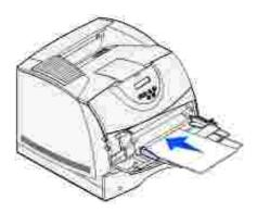
3. Slide the width guide to the left until it lightly touches the stack of print media. *Do not* bend the print media.
