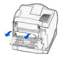
If the print media does not move immediately when you pull, stop pulling. Remove the toner cartridge, and then pull the print media out.
