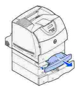
3. Pull the standard tray out of the printer.
