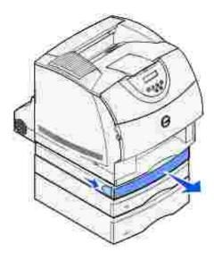
15. If the edge of the print media is visible, pull the print media straight up and out.
